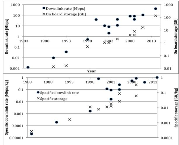
Fig. 1: Evolution of Downlink Rate & On-Board Storage in SSTL Delivered Satellites: 1.a) Absolute Value; 1.b) Specific Value
