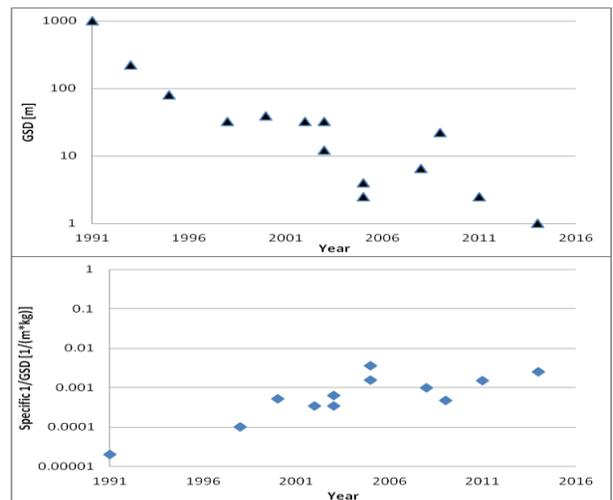
Fig. 2: Evolution of GSD in SSTL Delivered Satellites: 1.a) Absolute Value; 1.b) Specific Value
