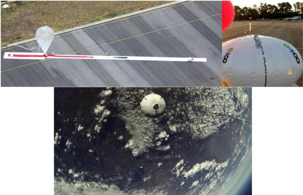
Figure 1: Stratospheric flight test of a multilayer flexible tank at 27km altitude
