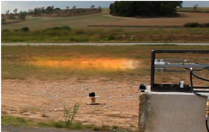
Figure 2: Static test of an early engine prototype
